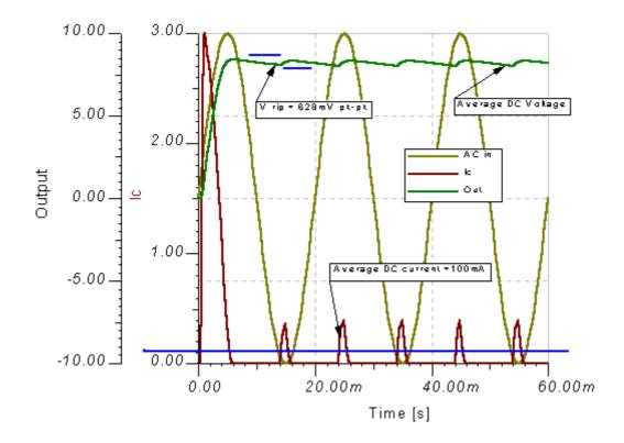
The calculated value of ripple is (0.1 \* 0.007) / 1000e-6 = 0.7 volts or 700mV. The value of peak-peak ripple measured from the graph is 628mV. Therefor, the equation is a good rule of thumb guide for choosing the correct value for a smoothing capacitor in a power supply.
